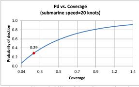
Fig.7. FFG's probability of detection as submarine speed=20 knots.
