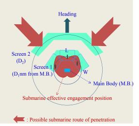
Fig. 3. Basic concept of convoy ASW design. (Source: United States Fleet Anti-Submarine Instructions)
